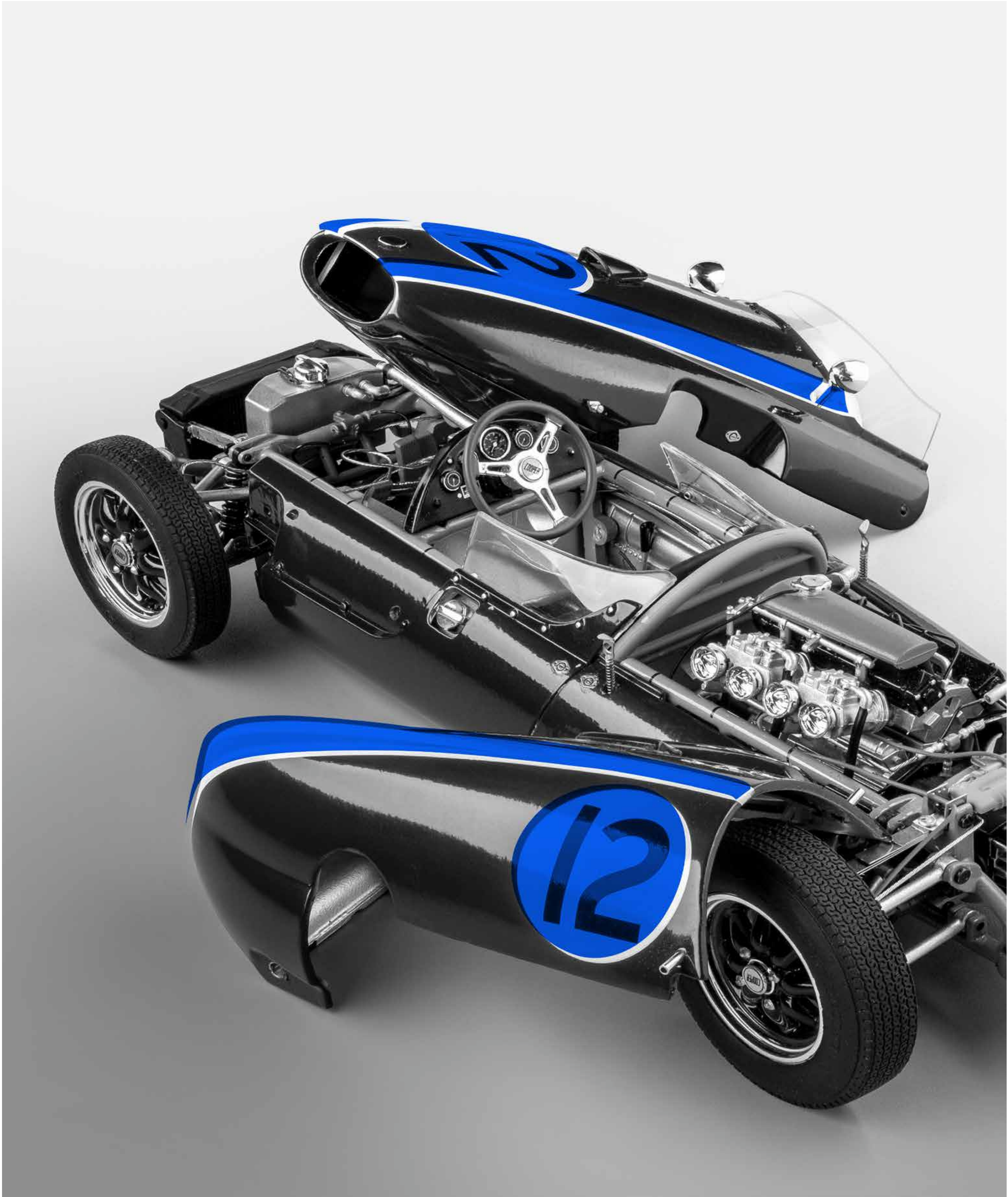
1959 COOPER CLIMAX T51 | 2,5L 4C | 240 HP | 6.750 RPM | 472 KG
