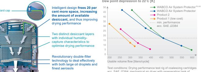
acc. SAE J2384; mechanical air dryer with regeneration tank of 6 liters, cut-in: 11 bar, cut-out: 12 bar
