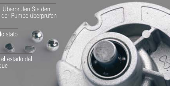
BROKEN BEARING ROULEMENT CASSÉ KAPUTTES LAGER CUSCINETTO ROTTO RODAMIENTO ROTO
